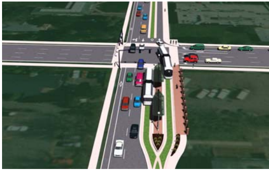
The high-speed corridor would incorporate characteristics such as signal priority and queue jumpers at intersections.
