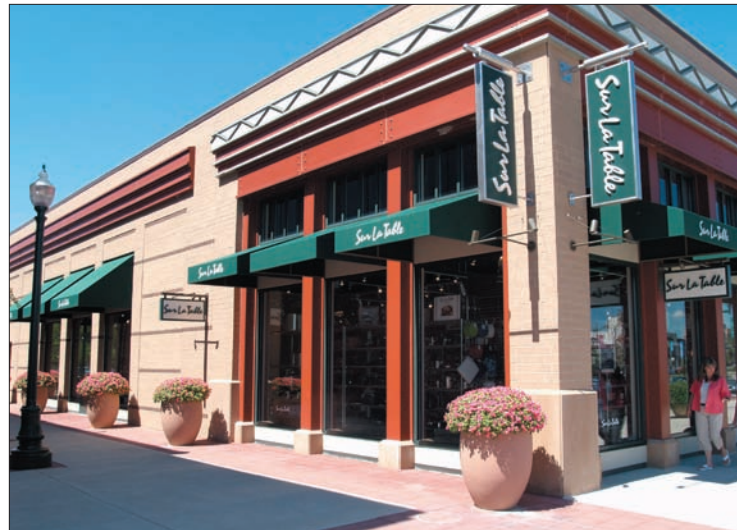
Building walls along streets should include at least 60% glass at ground level.
