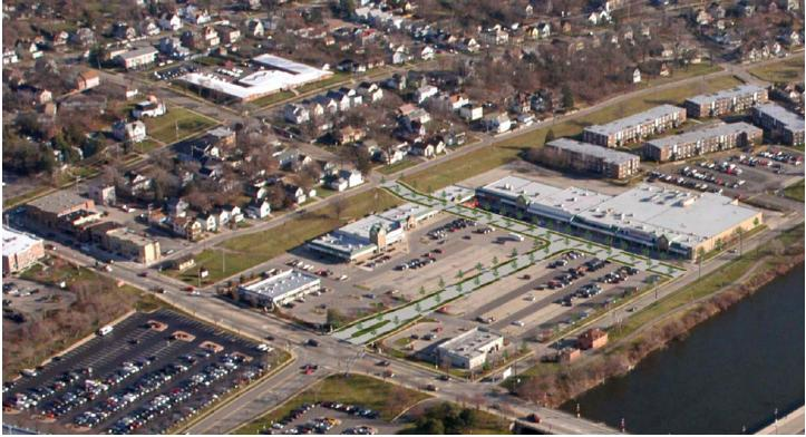
Phase 1: Remove a portion of the storefront, and extend Watch Street through, aligning with the front of the existing Butera Grocery Store, and "T" into Times Square Road. Extend Grove Avenue south to intersect with the newly constructed Watch Street roadway.
