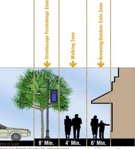
Figure 4.2: Sketch showing the sidewalk zones
