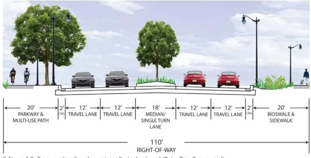
Figure 1.8: Cross-section though a major collector boulevard (Outer Ring Commercial)
