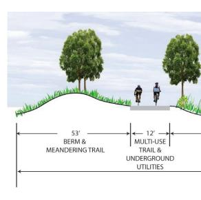
Figure 1.6: Cross-Section through the Elgin-O'Hare Boulevard -
