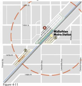
In Phase 2, the existing Parking Lots 3 and 7 will be reconstructed along with the property between these two lots into an expansion of the Parking Lot constructed in Phase 1 Parking Lot A. Lot A will house parking spaces displaced by this construction. This expanded lot will be large enough to hold all parking spaces that are currently in Parking Lot 2 in order to free this area up for the construction of the Village Green.
