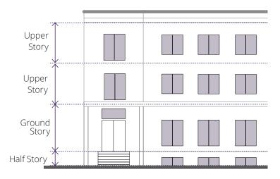
Figure 9-4D-28. Measuring Minimum Facade Transparency per Story
