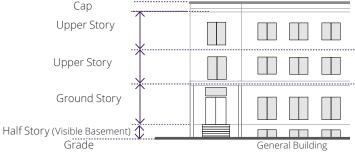
Figure 9-4D-26. Measuring Stories with Floor-to-Floor Height
