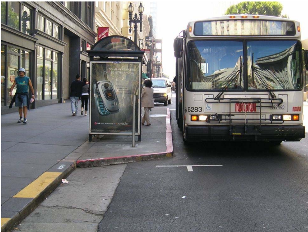
Figure 17: Example of a Bus Bump Out
