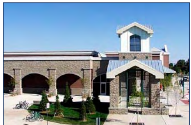
❖ Blank walls should be avoided; if necessary facade modulation, such as these arched overhangs and columns should be utilized to enhance appearance.
