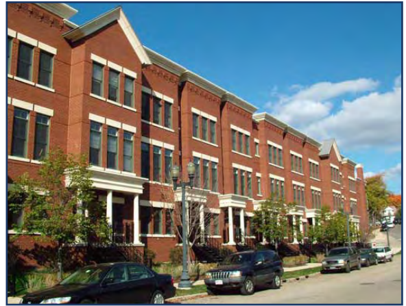
❖ Building entrances are defined by columns, cornice overhangs and stairs leading up to each unit.
