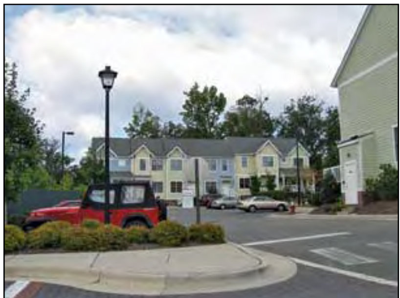
❖ Landscaped parking islands increase the amount of pervious surface on-site, allowing for improved stormwater drainage. Plantings also screen cars and service areas.
