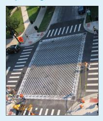
Define crosswalks by incorporating alternative paving materials (above), and provide bumpouts (below) at corners where they will not interfere with bus movement.
