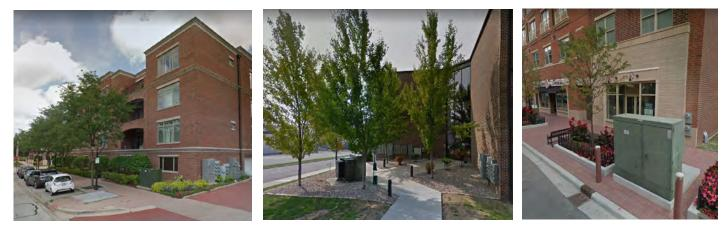
Figure 5-N. Examples of Poorly Located Utility Appurtenances without Screening on Primary Streets: NOT PERMITTED
