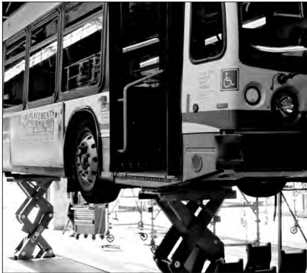
CTA is repairing and replacing hoists at its seven bus facilities that are either non-functioning or beyond their useful life. The repairs, which will continue through 2014, will provide a safer and more efficient work environment.
