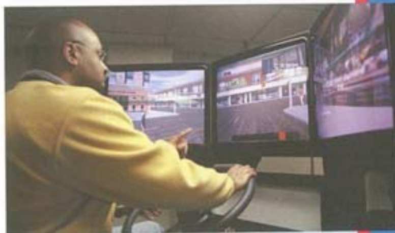
CTA's new bus simulator recreates driving conditions to prepare operators for service in the real world.
