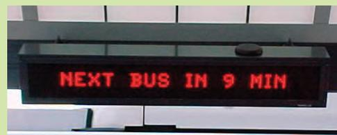
Real time passenger information displays at bus stops and transfer centers provide passengers with reassurance on the time they will have to wait for their bus.
