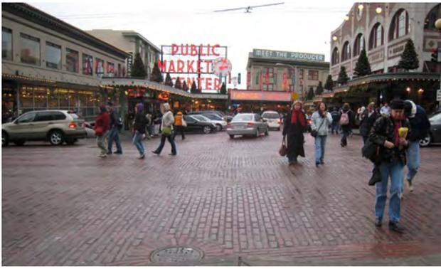
A pedestrian-only phase in the signal at Pike Place Market in Seattle allows pedestrians to cross in all directions while cars are stopped. Special brick pavement through the intersection provide a visual and tactile reminder of the crosswalk. Vehicles cannot turn right during a red light at this intersection, so pedestrians are free to cross with less threat of being hit by a turning car.
