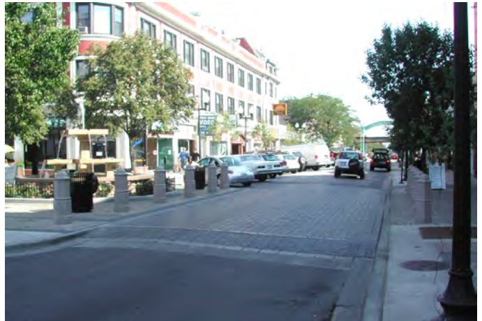
Pedestrian crossing zones can be distinguished by raised paving and/or a distinct paving pattern.
