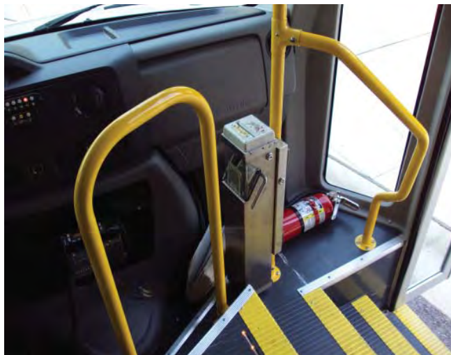
This fare drop box is installed on all paratransit vehicles in the suburbs.
